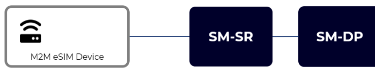
SGP.01 eSIM Architecture for M2M
